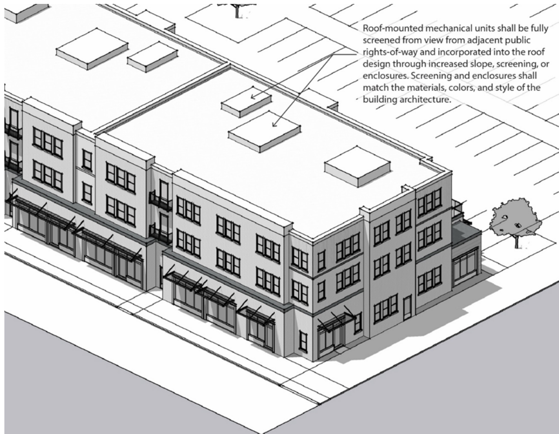
Fig. 9: Roof Mounted Mechanical Units
