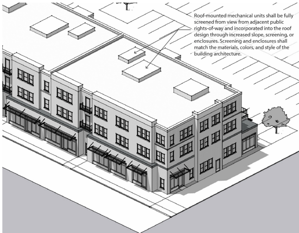
Fig. 9: Roof Mounted Mechanical Units
